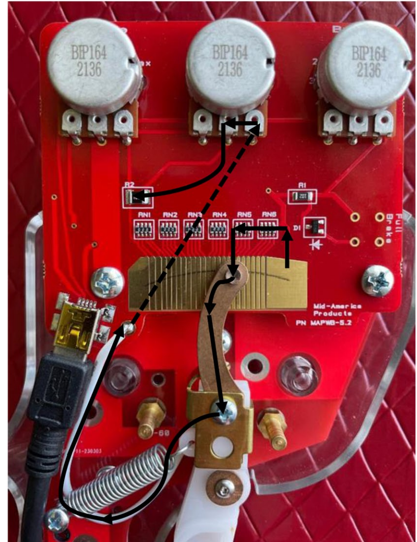
Figure 7. Wiper Board Current Flow – Curved Response
