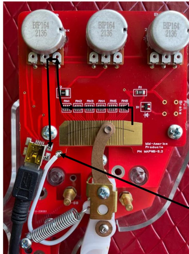
Figure 2. Wiper Board Current Flow – Partial Throttle
