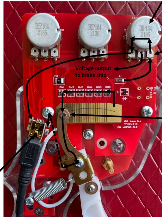
Figure 5. Troubleshooting Steps – Brake Circuit
